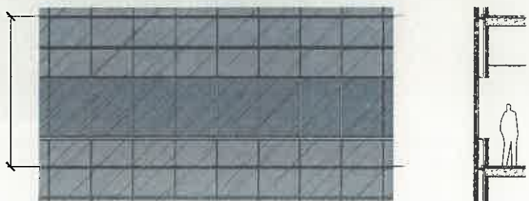
ASSEMBLY 4 Curtain-wall facade Marina Bay model Vision glazing 24mm-thick double glazed units—glass layers 6mm thick each Spandrel glass Single-glazed 8mm thick
