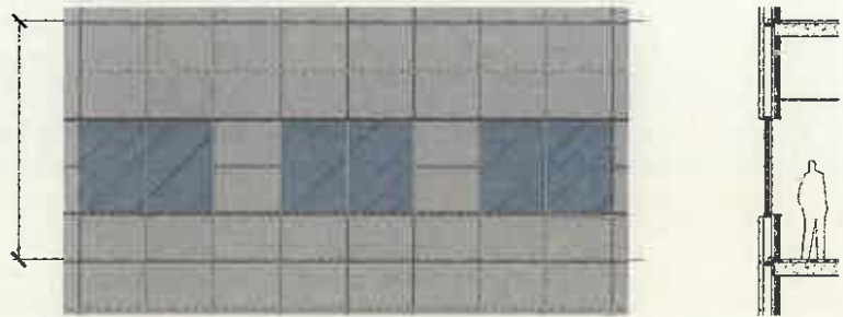
ASSEMBLY 2 Granite slab-clad facade Marina Centre model (with individual windows to represent actual circumstances in Marina Centre) Granite thickness 25mm Vision glazing 24mm-thick double glazed units—glass layers 6mm thick each
