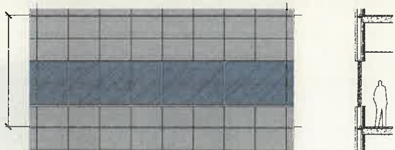
ASSEMBLY 3 Aluminium-clad facade Marina Centre model Aluminium panel thickness 3mm Vision glazing 24mm-thick double-glazed units—glass layers 6mm thick each
