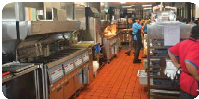
The Low Oil Volume (LOV) fryer uses less oil and is more energy-efficient.
